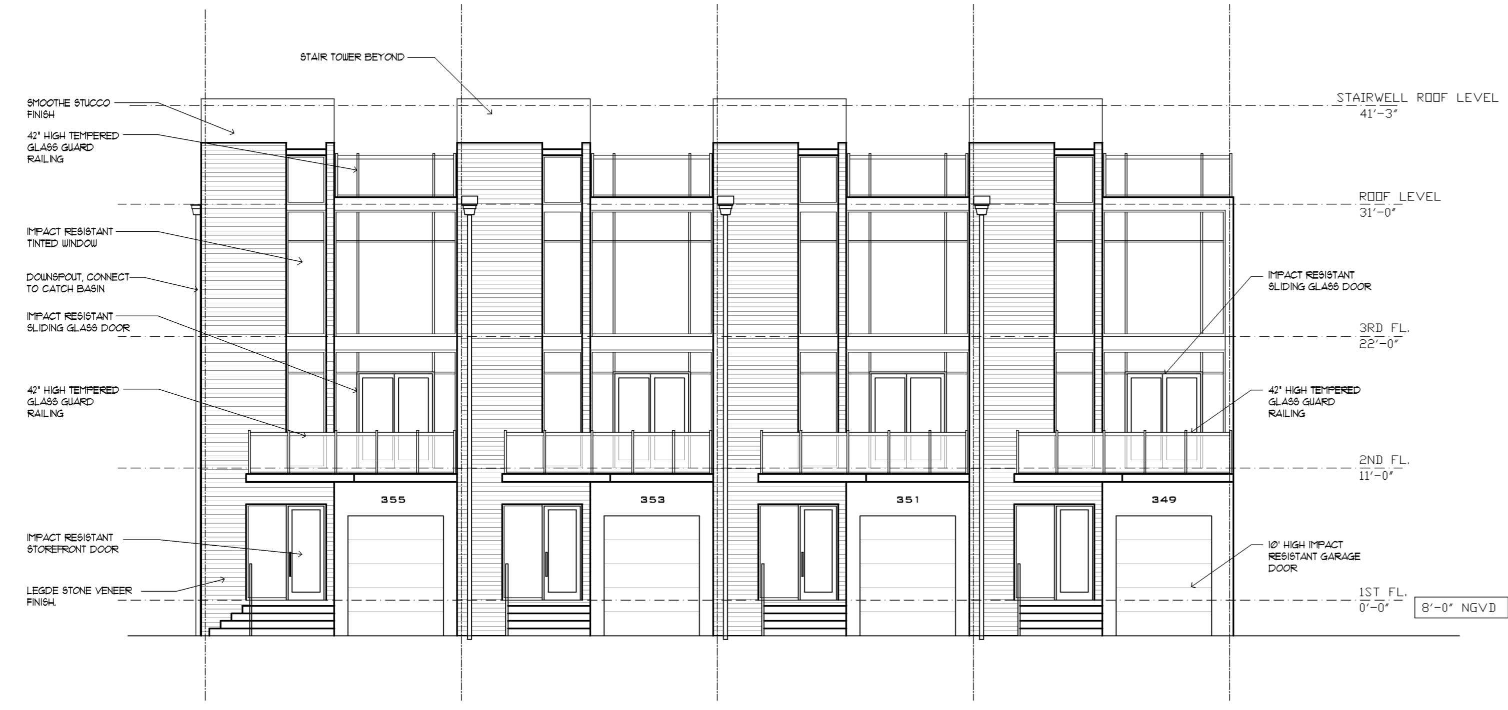
SOUTH ELEVATION PALM STREET
